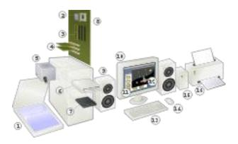
Basic hardware components of a modern personal computer, including a monitor, a motherboard, a CPU, a RAM, two expansion cards, a power supply, an optical disc drive, a hard disk drive, a keyboard and a mouse
