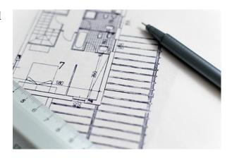
A floor plan is copied for each of the trades that will be involved in the construction of the building. For example, there is an electrical floor plan, a plumbing floor plan, an HVAC (heating, ventilation, and air conditioning) floor plan, etc.
